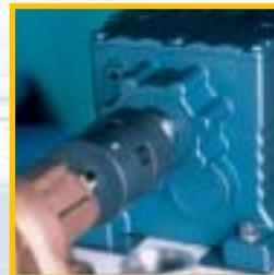
Static build-up on a motor shaft found its way to ground through the bearing, pitting and shortening the life of the rolling elements. A unique additive package worked synergistically to create an electron pathway through the grease to reduce pitting and extend bearing life.
