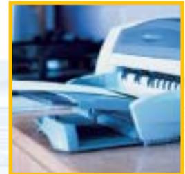
Gears in the paper feed mechanism of an office printer were too noisy to meet quality specs. Increasing the viscosity of the PAO base oil eliminated unwanted noise and extended gear life.
