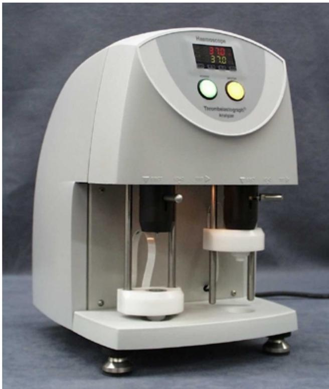
Thrombelastograph® (TEG®) Coagulation Analyzer, manufactured by Haemoscope Corporation of Skokie, Ill., tracks the shear elasticity of a clot and its ability to arrest bleeding — in real-time, during a medical procedure. It relies of two greases by Nye Lubricants, one in the gear motor and one where mating parts slide on the frame.
