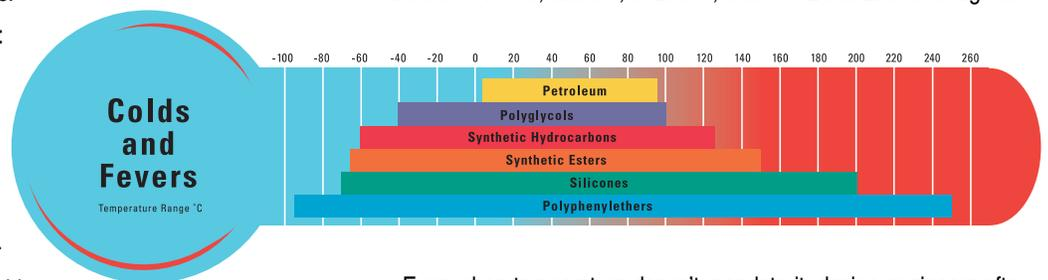
Even when temperature doesn't mandate it, design engineers often choose a synthetic lubricant. Compared to petroleum, synthetic oils are more chemically homogeneous. They offer better thermooxidative stability. Oxidation not only depletes lubricant supply, it often leaves abrasive oxides in its wake — which hastens component failure. At elevated temperatures, even without the presence of oxygen, synthetic lubricants are also less volatile than petroleum-based products of equivalent viscosity.
