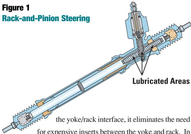
the yoke/rack interface, it eliminates the need for expensive inserts between the yoke and rack. In addition, the grease allows for greater tolerances when securing the yoke plug.
