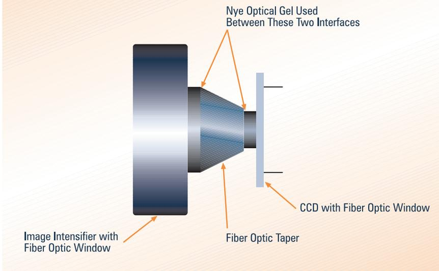
**Figure 2: Non-Curing Optical in Image-Intensified CCD Camera**
