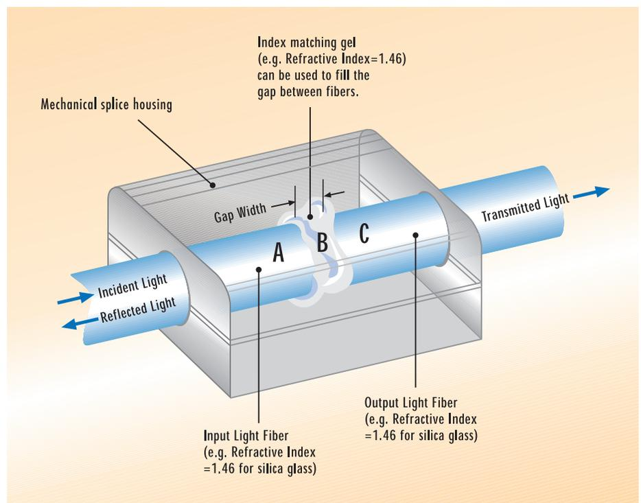
**Figure 1: Basic Configuration of a Fiber Optic Mechanical Splice**
