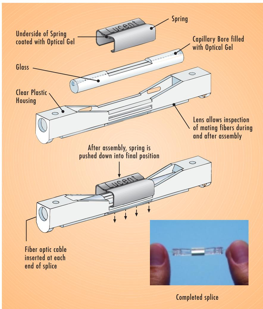
**Figure 3 – Illustration of Lucent's CSL LightSplice**
