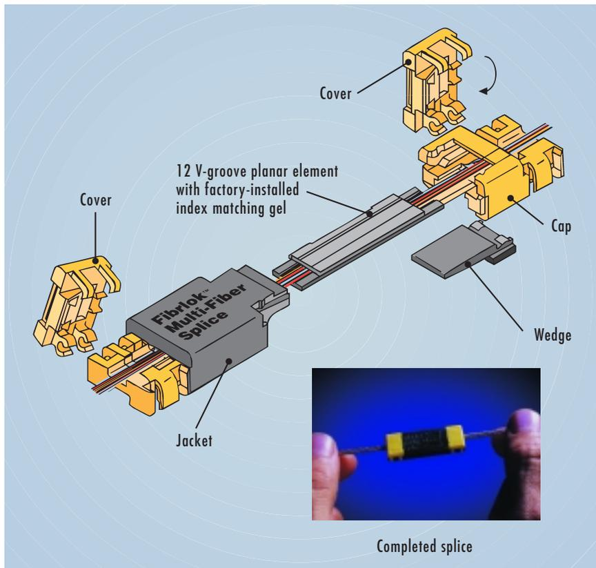
**Figure 2 – Illustration of 3M's Fibrlok™ Splice**
