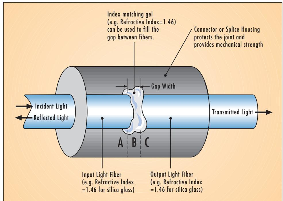
**Figure 1 – Basic Configuration of a Fiber Optic Interconnect**
